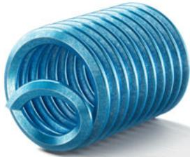
The new thread insert merges the advantages of the HELICOIL® Plus and the HELICOIL® Tangfree. Every thread of the thread insert with precision-formed, rhombic profile is free running. The result is a true-to-gauge internal thread including the last thread which is in every case threadable.
