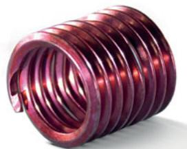
HELICOIL® Tangfree Screwlock has the same advantages as HELICOIL® Tangfree. In addition, there is a screw-locking area. The screw is locked by one or several polygonal-shaped threads clamping the flanks of the screwed in screw. The elastically resilient frictional locking results in prevailing torques similar to the specifications of ISO 2320. These screw locking torques meet the demands of technical delivery terms regarding international standard specifications.
