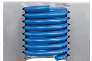
Correct installation of HELICOIL® Smart ( $0.25 - 0.5 \times P$  below the surface of component)
