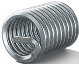
Every thread of the thread insert with precision-formed, rhombic profile is free running. The result is an internal thread true to gauge that can be used from both ends. The dimensional stability of the ISO thread complies with DIN 13 6H as well as for special requirements with 4H and meets the demands on international standard specifications.
